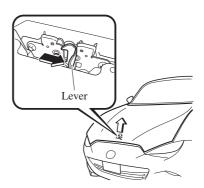
Grasp the support rod in the padded area and secure it in the support rod hole indicated by the arrow to hold the bonnet open.
