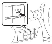
By pressing the switch until a beep sounds, the i-stop function is turned off and the i-stop warning light (amber) in the instrument cluster turns on. By pressing the switch again until the beep sounds, the i-stop function becomes operational and the i-stop warning light (amber) turns off.
