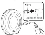
11. Hold the bottom of the bottle upright, squeeze the bottle with your hands, and inject the entire amount of tyre sealant into the tyre.
