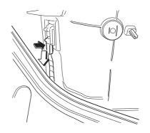
4. Pull the centre of each plastic retainer and remove the retainers, and then partially peel back the boot side trim.
