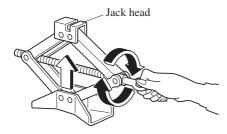
4. Place the jack under the jack-up position closest to the tyre being changed with the jack head squarely under the jack-up point.
