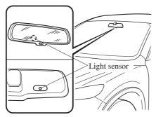
The auto-dimmer function is cancelled when the ignition is switched ON and the shift/selector lever is in reverse (R).
