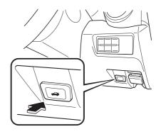
The remote release button function can be disabled by locking the doors using the transmitter, auxiliary key, or a request switch to prevent an intruder in the vehicle from opening the boot.
