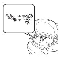
Partially peel back the cover inside the boot, then pull the emergency release lever.
