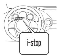
• The i-stop indicator light (green) turns off when the engine is restarted.
