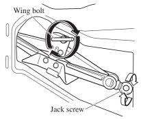
3. Turn the wing bolt completely to secure the jack.
