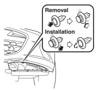
Turn the screw anticlockwise and remove it, and then partially peel back the mudguard.
