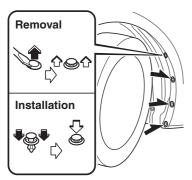
Remove the unit by pressing the tab on the unit with your finger and pulling the unit forward.
