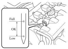
5. Pull it out again and examine the level. The level is normal if it is between Low and Full.
