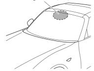
The Forward Sensing Camera (FSC) determines the conditions ahead of the vehicle while travelling at night and detects traffic lanes. The distance in which the Forward Sensing Camera (FSC) can detect objects varies depending on the surrounding conditions.
