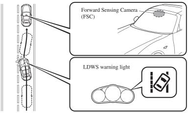
The warning light illuminates when the system has a malfunction. Refer to Warning Lights on page 4-32.
