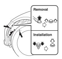
Disconnect the connector from the unit by pressing the tab on the connector with your finger and pulling the connector rearward.
