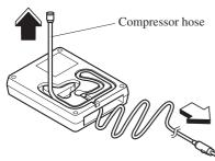
17.Install the air compressor hose to the tyre valve.
