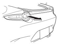
7. Turn the socket and bulb assembly anticlockwise and remove it.
