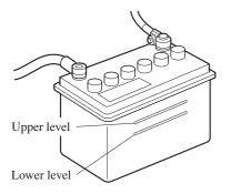
Inspect the electrolyte level at least once a week. If it is low, remove the caps and add enough distilled water to bring the level between the upper and lower level (illustration).
