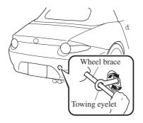
4. Hook the towing rope to the towing eyelet.
