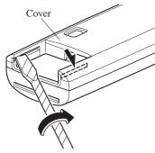
3. Insert the tape-wrapped flathead screwdriver into the gap and slide it in the direction of the arrow.
