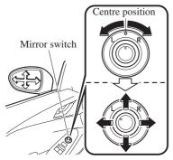
After adjusting the mirror, lock the control by rotating the switch to the centre position.
