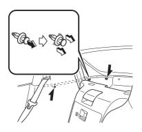
4. Partially peel back the cover on the right side of the vehicle.
