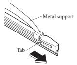
Remove the metal stiffeners from each blade rubber and install them in the new blade.
