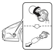
6. Install the new bulb in the reverse order of the removal procedure.
