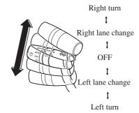
The direction indicators (green) in the instrument cluster flash according to the operation of the direction indicator lever to show which signal is working.
