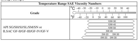
Engine oil viscosity, or thickness, has an effect on fuel economy and cold-weather operation (starting and oil flow).
