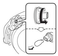
7. Install the new bulb in the reverse order of the removal procedure.
