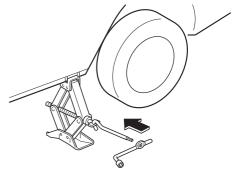
7. Turn the jack handle clockwise and raise the vehicle high enough so that the tyre is raised off the ground and can be removed. Before removing the wheel nuts, make sure your Mazda is firmly in position and that it cannot slip or move.
