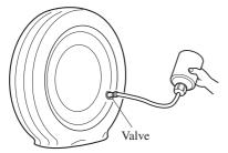
12.Pull out the injection hose from the valve.
