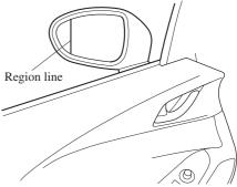
• The perceived distance of objects in the outer and inner regions of the wide angle mirror is different. Objects appearing in the outer region are actually further away than they are in the inner region.
