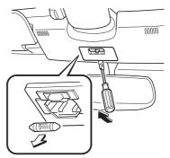
3. Install the new bulb in the reverse order of the removal procedure.
